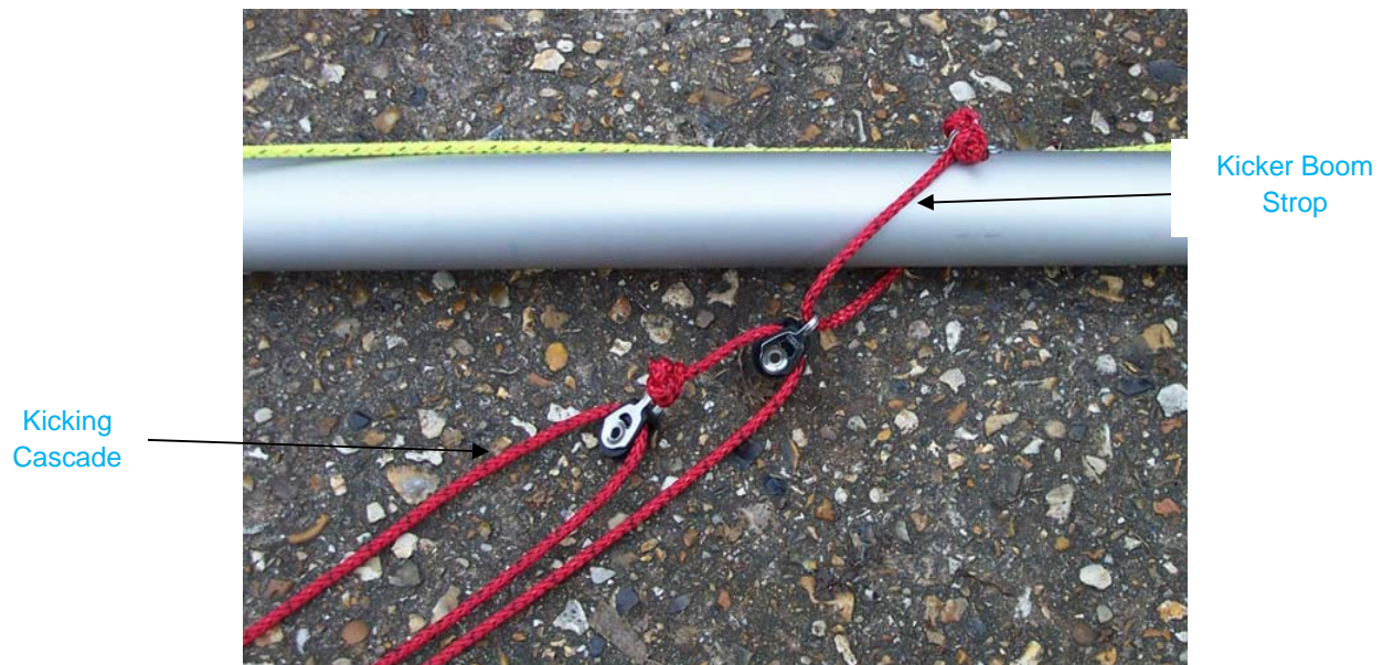
Picture 4.14 The Kicking Cascade Attached
