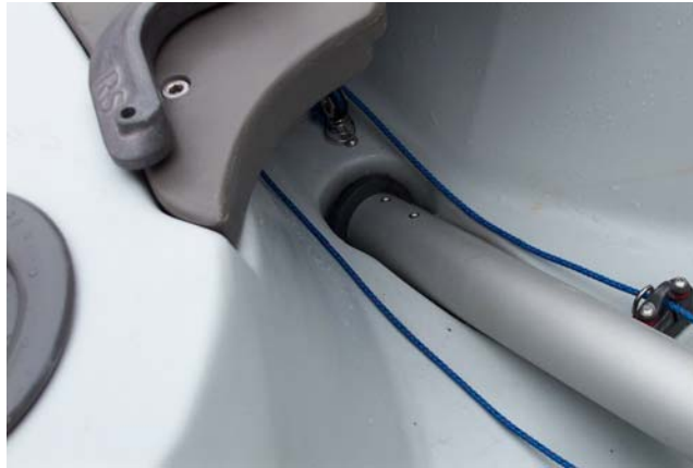
Picture 4.10 The Mast Foot in the Mast Well
