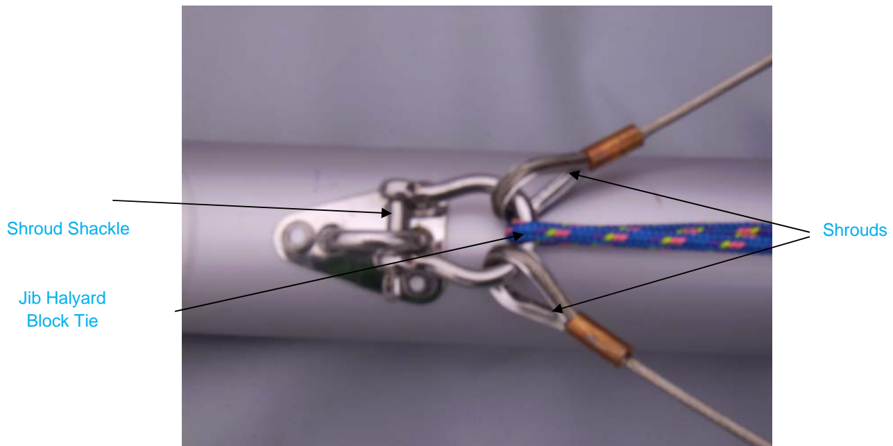
Picture 4.24 Fixing the Shrouds
