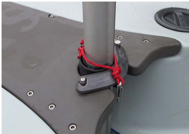
Picture 4.11 The Mast Up With the Mast Gate Closed
