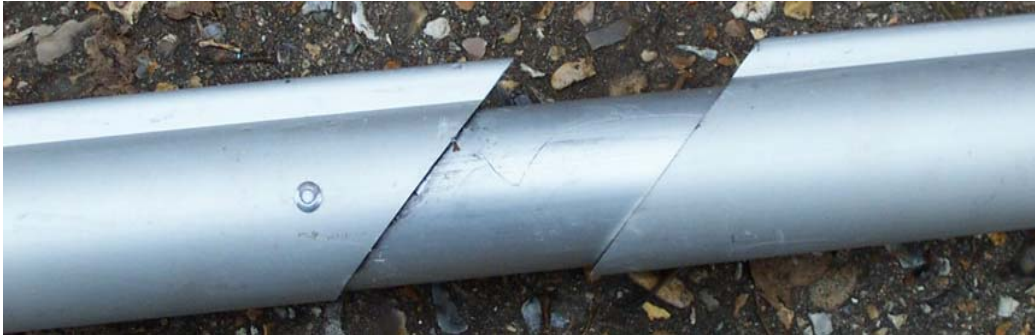
Picture 4.5 Joining the Mast
