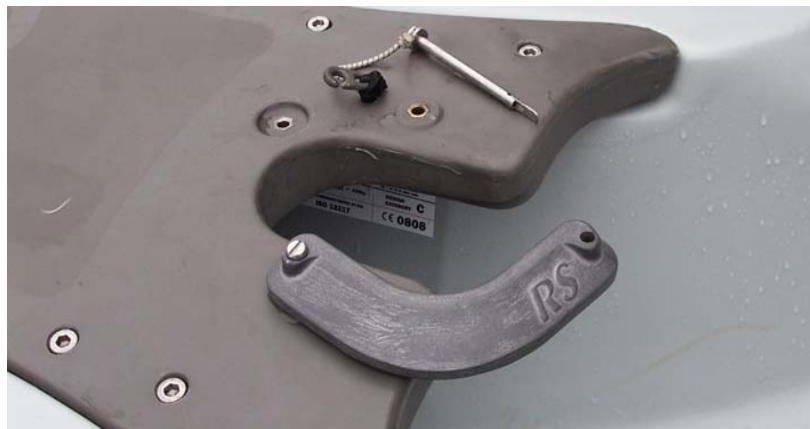
Picture 4.9 The Open Mast Gate
