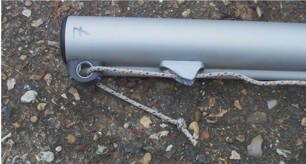
Picture 4.7 Threading the Main Halyard
