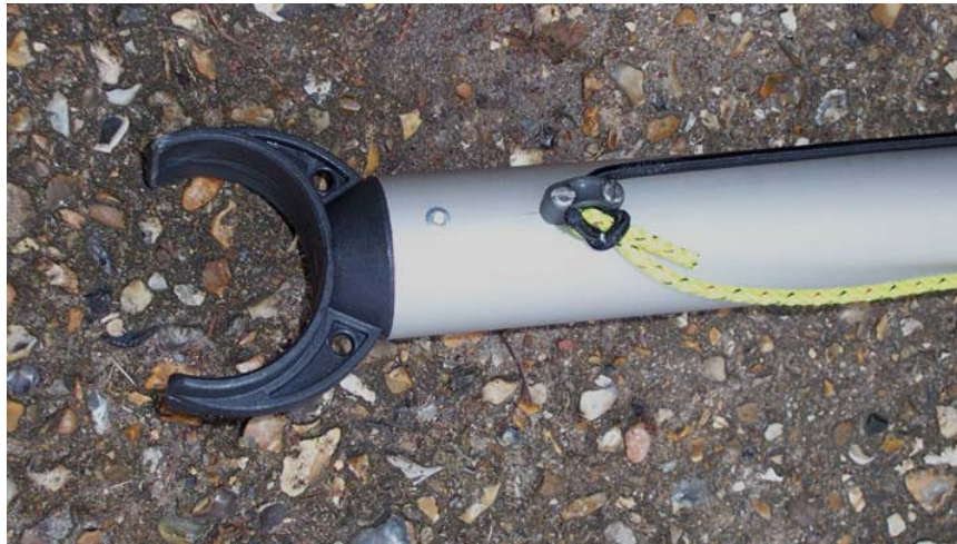
Picture 4.13 The Front End of the Boom and the Gooseneck
