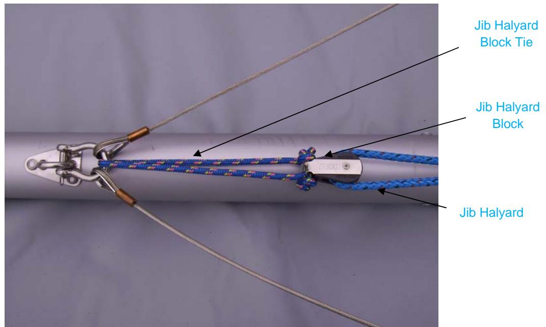
Picture 4.25 Rigging the Jib Halyard Block
