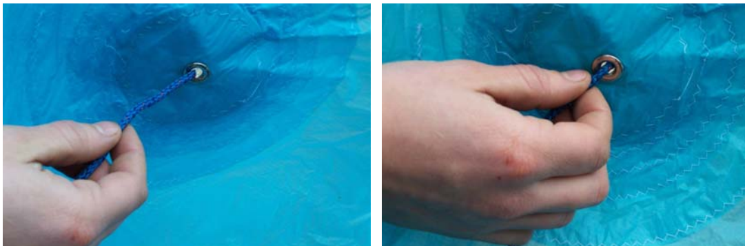
Picture 4.31 Threading the Gennaker Downhaul Line
