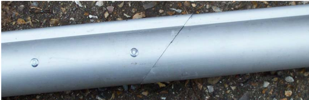
Picture 4.6 A Joined Mast
